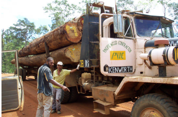
Plate 11 Jinker driven with no safety chain.
